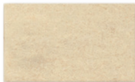
Neu-Filz 219 white density 0.25-0.40 g/cm 3 thickness 1-30 mm
