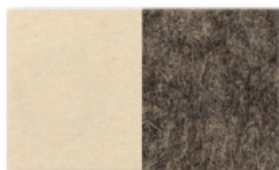
Neu-Filz 1004 white/2002 mottled density 0.50-0.68 g/cm 3 thickness 5-30 mm
