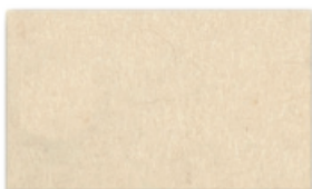
Neu-Filz 205 white density 0.41-0.49 g/cm 3 thickness 1-10 mm
