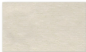
Neu-Filz 285 white density 0.18-0.20 g/cm 3 thickness 1-10 mm
